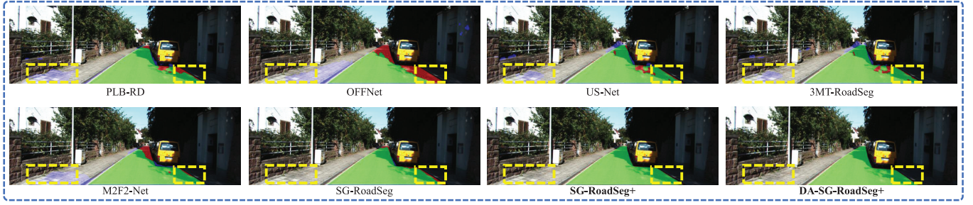
Fig. 6. Qualitative comparison between our proposed SG-RoadSeg+ and other SoTA feature-fusion networks on the KITTI Road [33] dataset. The true positive, false negative, and false positive pixels are shown in green, red, and blue, respectively.
