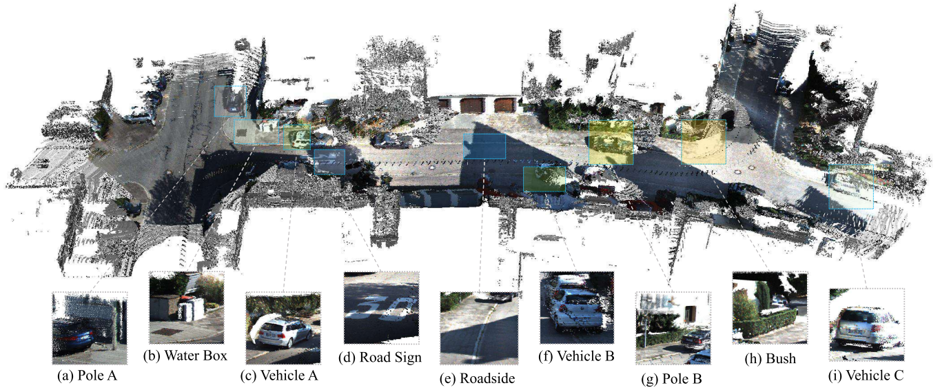
Fig. 1. Visualization of calibration results through LiDAR and camera data fusion in KITTI odometry 00 sequence: (a)-(i) zoomed-in regions that illustrate the alignment between the camera images and the LiDAR point clouds.
