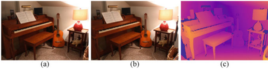
Fig. 3.17 Example images of middlebury 2014 dataset [15]. a Left stereo image; b right stereo image; c ground truth disparity map
