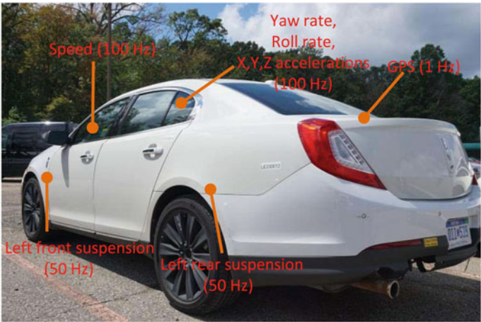
Fig. 11.4 In-vehicle sensors for vibration signals collection [27]
