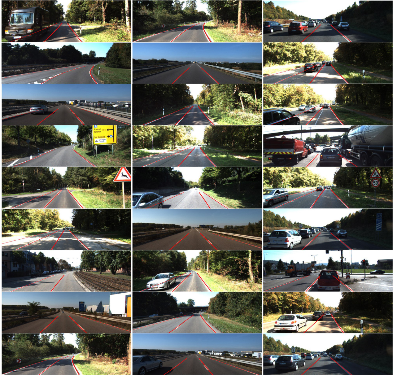
Figure 9. Lane detection results. The red lines illustrate the detected lanes.
