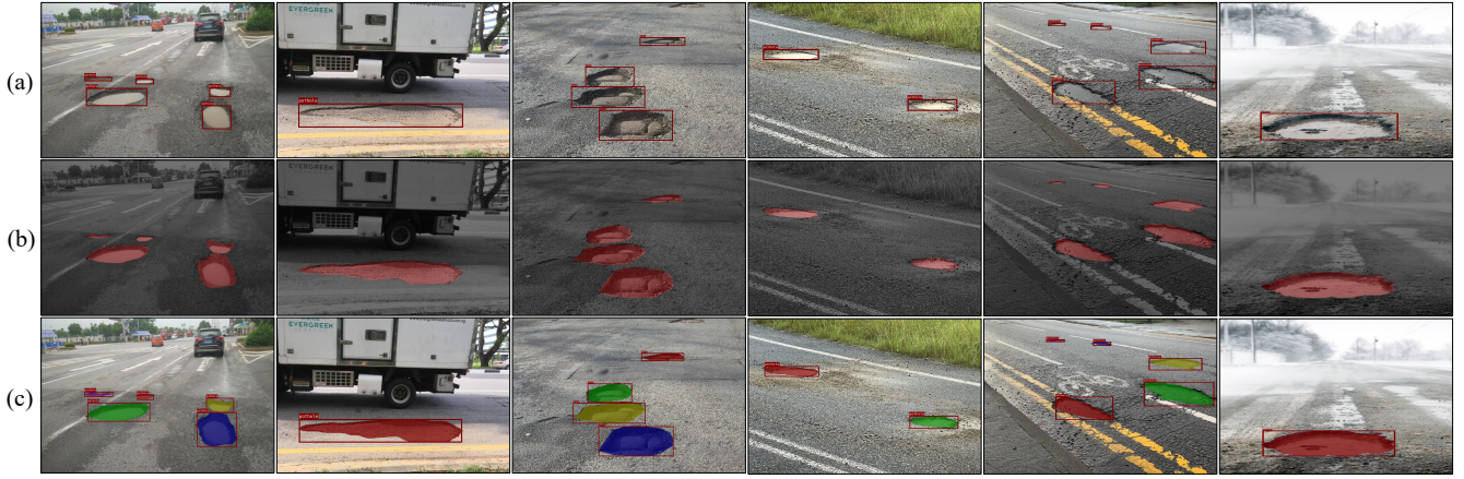
Fig. 3. Examples of the UDTIRI dataset: (a) object detection annotations; (b) semantic segmentation annotations; (c) instance segmentation annotations.
