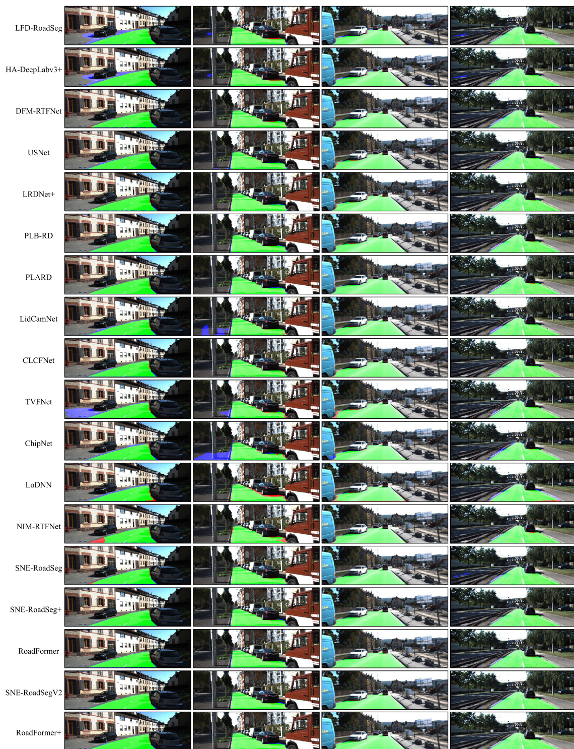
Figure 5 Qualitative comparisons of SoTA road scene parsing networks on the KITTI Road dataset [29], with true-positive, false-positive, and false-negative classifications shown in green, blue, and red, respectively
